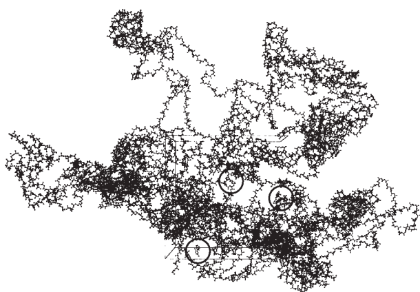
Figure 8 Typical conformation of iPP/UVA-2 blends with five chains of iPP (MM : 50,000) and three molecules of UVA-2 per unit cell.
